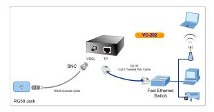
Figure 3-5: Connecting Multiple PCs to an Ethernet LAN
